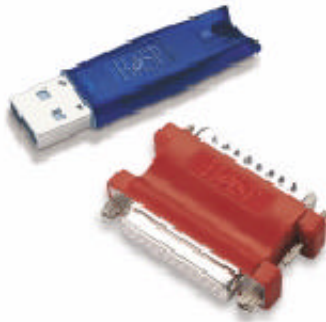
Figure 9: USB and parallel port dongles, which contain a sufficient amount of memory to store an encrypted secret key. The example certificate management scheme uses the AES symmetric encryption algorithm to encrypt an SA’s secret key using a pass-phrase supplied by the SA, and then writes it into the dongle for portability and easy use. Image source: Aladdin Knowledge Systems Ltd.
